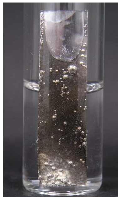
Fig. 3 Photographs showing the reaction of Al substrate in the aqueous solution of pH 11.6
